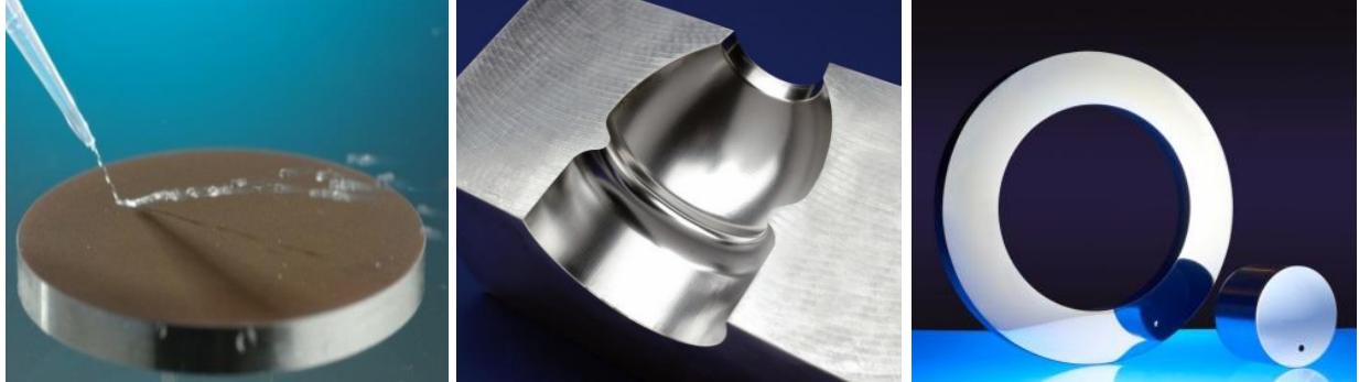
Figure 1: left: laser structured hydrophobic surface, middle: laser polished blow mould, right: automotive parts with laser functionalised thin-films for wear protection
