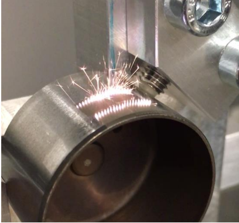
Figure 9: Laser structuring of a part provided by an end-user in the project using the multi-beam optics integrated in the developed machine tool
